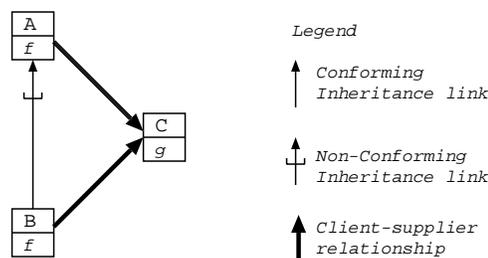
**Figure 3:** The method **f** of the class **A** uses the method **g** of the class **C**. When **f** is NC-inherited by **B**, it should still be allowed to use **g**.
