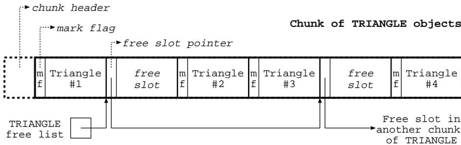
Figure 2: Detail of a fixed-size object chunk
